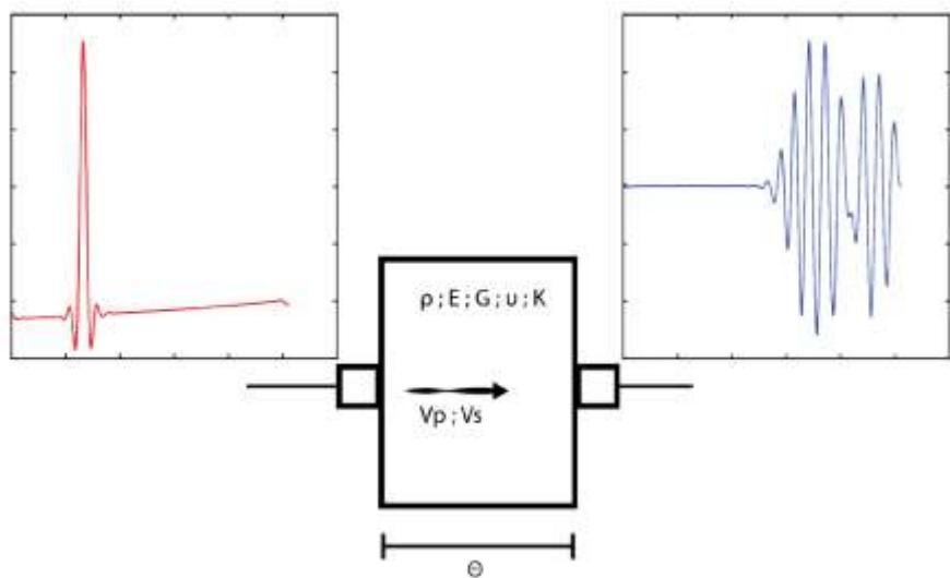
The transducers consist in elements that convert electrical pulses into mechanical pulses and vice-versa. Piezoelectric elements were used in this example. A piezoelectric element contains ceramics or crystals whose vibrations will perform the conversion task.
